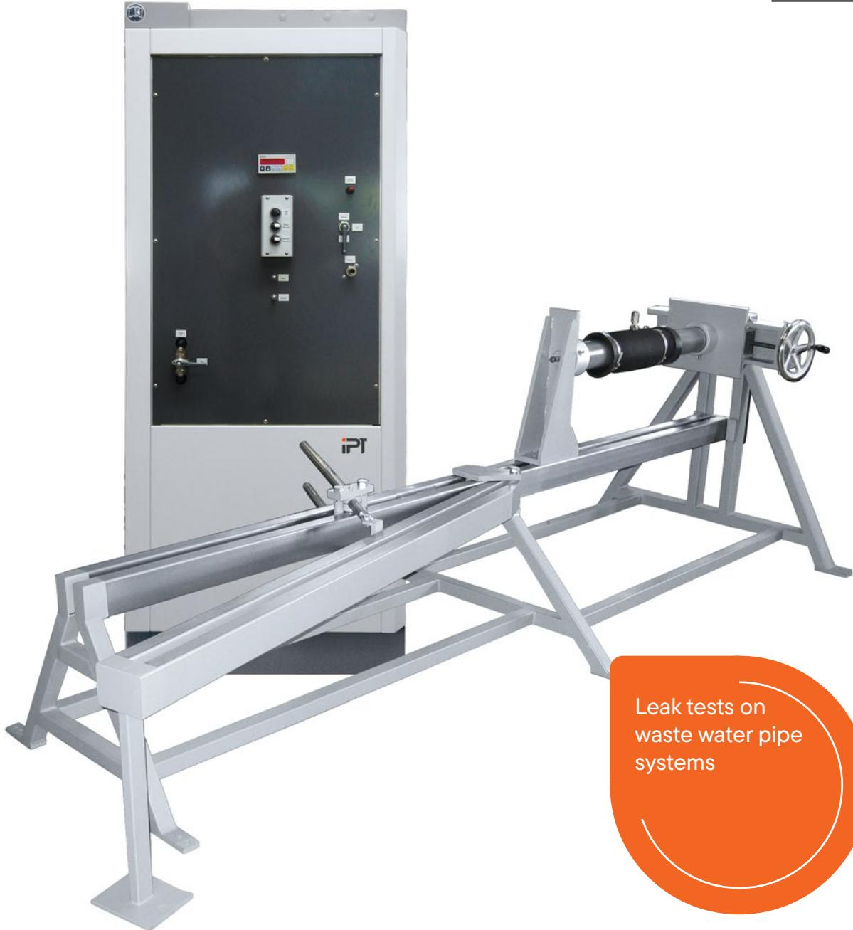
The combi test stand 1351 is used to carry out leak tests on waste water pipe systems in the diameter range DN 40 to DN 400. The modular design allows for step-by-step expansion in order to apply additional load types.
