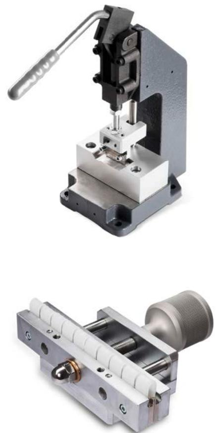
**ASTM D1693 Standard Test Conditions**
