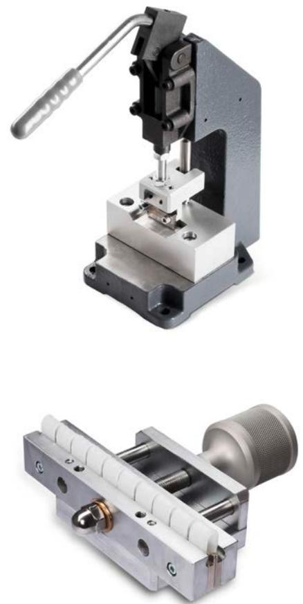
**ASTM D1693 Standard Test Conditions**
