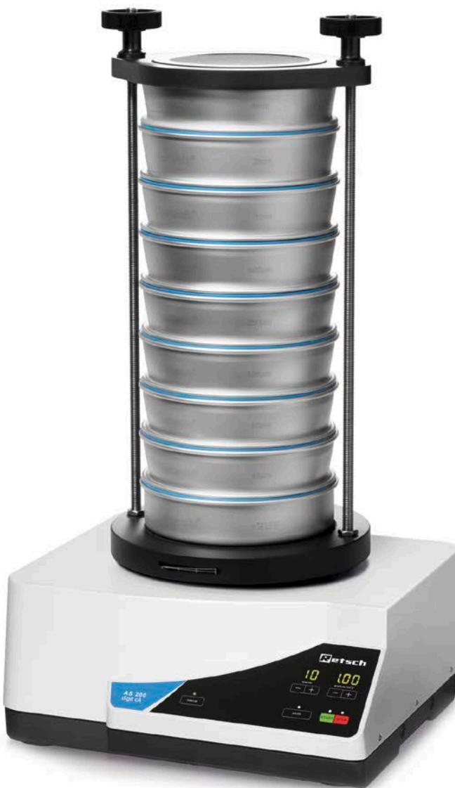
The digital sieving machine allows you to easily and precisely determine the fineness and grain size distribution of all powder or grain-like products. The material to be sieved is moved in a 3-dimensional circular motion in the 8 sieves and sieved according to the relevant test specifications with respect to the vibration level, time and interval. The results are fully reproducible for dry sieving. Operation is
