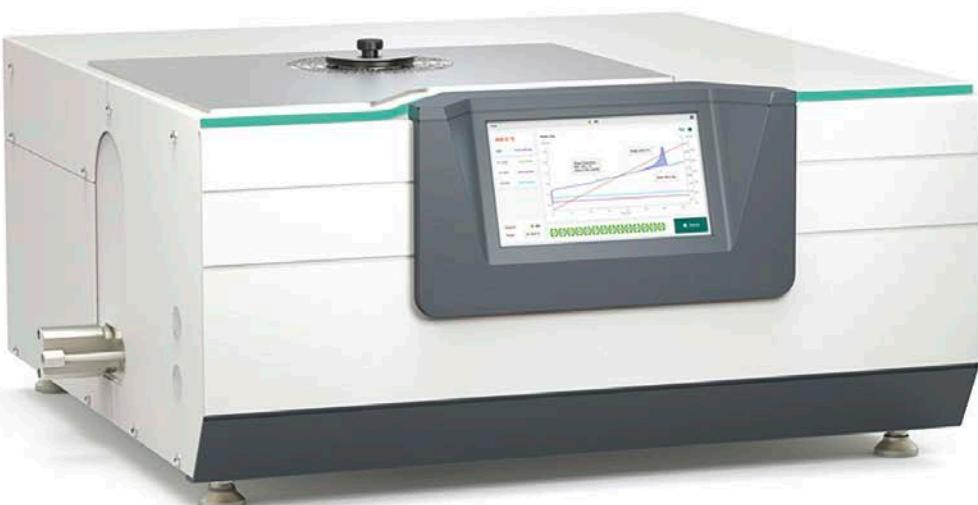
Dynamic differential calorimeter for determining the oxidation induction time for plastic piping and protective pipe systems, as well as fittings made of polyolefins. The period of time during which an antioxidant remains in the specimen and thus prevents oxidation is measured. For testing, the material sample is kept in flowing oxygen at a constant, specified temperature. The dynamic differential calorimeter
