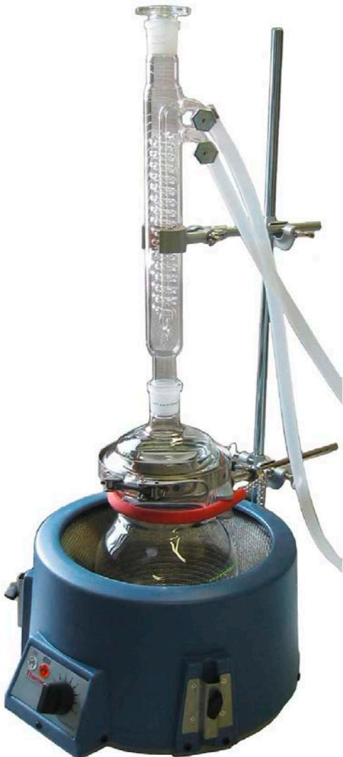
ISO 10147 stipulates that test samples made from crosslinked polyethylene (PE-X) must be stored in a specified, boiling solvent for a specific period of time and that the percent by weight of insoluble material is then measured. The percentage of insoluble material must be recorded to express the degree of crosslinking. For this
