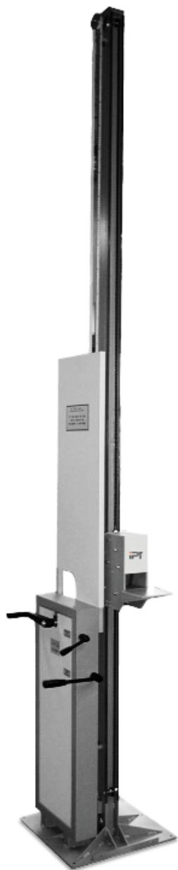
You can test packaging of varying shapes and sizes for impact stress after free fall using IPT's drop testers. The packaging can be tested with its content and may consist of cans, barrels and boxes. The holding device on the platform
