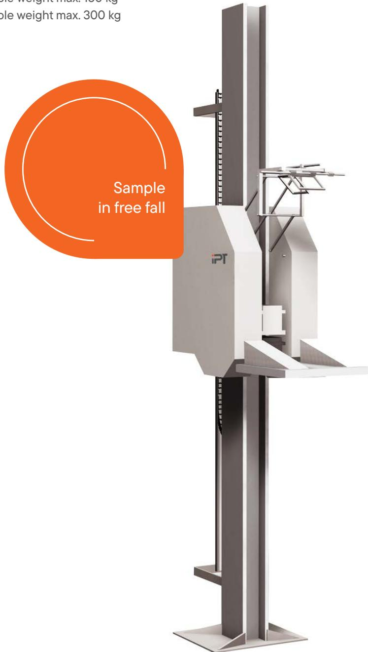
You can test packaging of varying shapes and sizes for impact stress after free fall using IPT's drop testers. The packaging can be tested with its content and may consist of cans, barrels and boxes. The holding device on the platform
