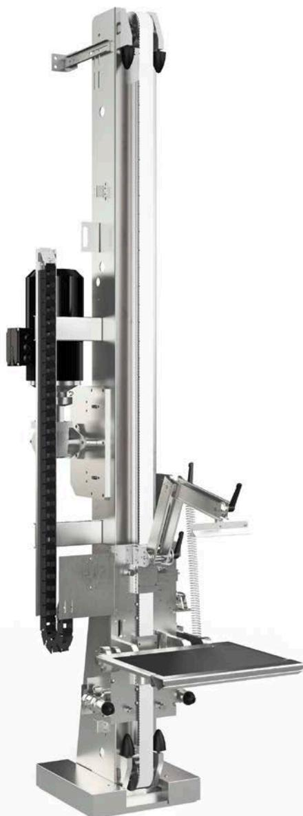
You can test packaging of varying shapes and sizes for impact stress after free fall using IPT's drop testers. The packaging can be tested with its content and may consist of cans, barrels and boxes. The holding device on the platform holds the sample in various drop positions. As the platform
