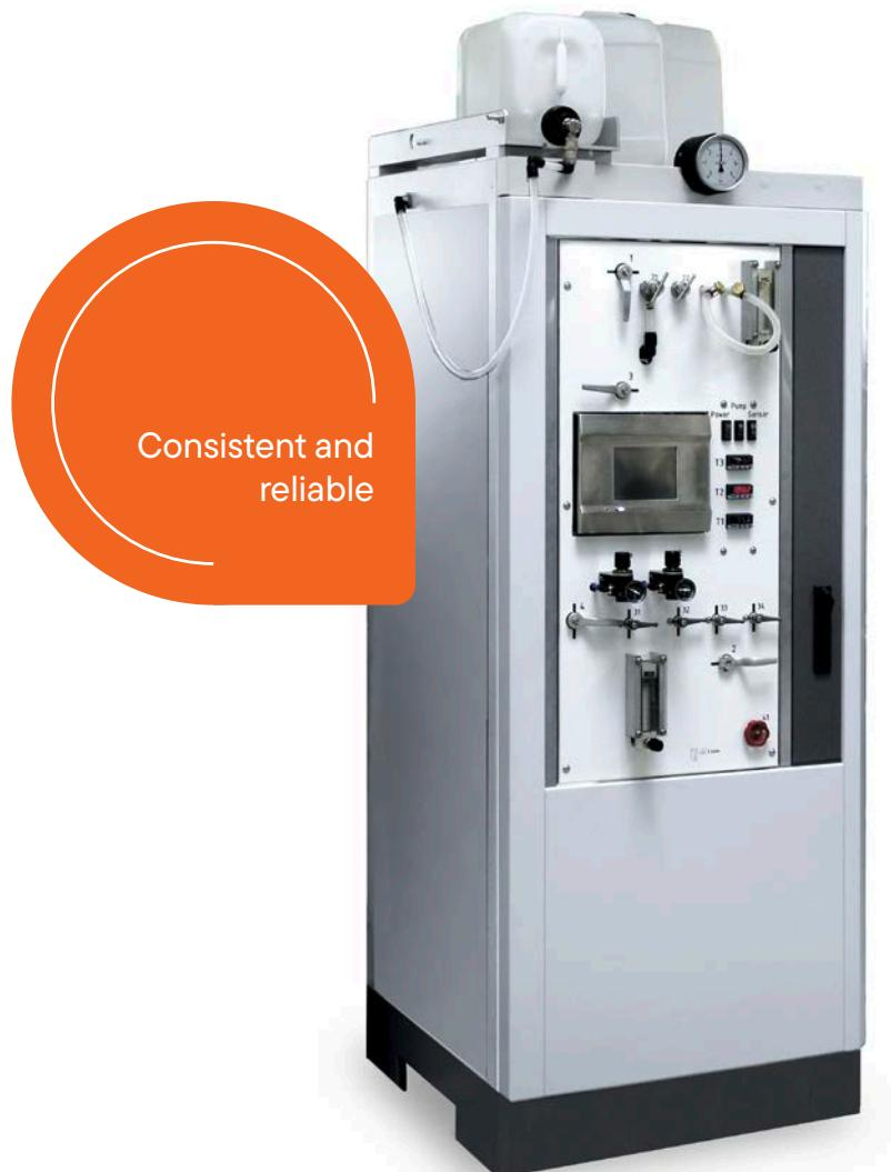
This testing device is used to determine oxygen diffusion through the pipe wall of composite pipes. The testing device consists of a supply unit (built into an installation frame), a hot air oven and a drum for holding the test
