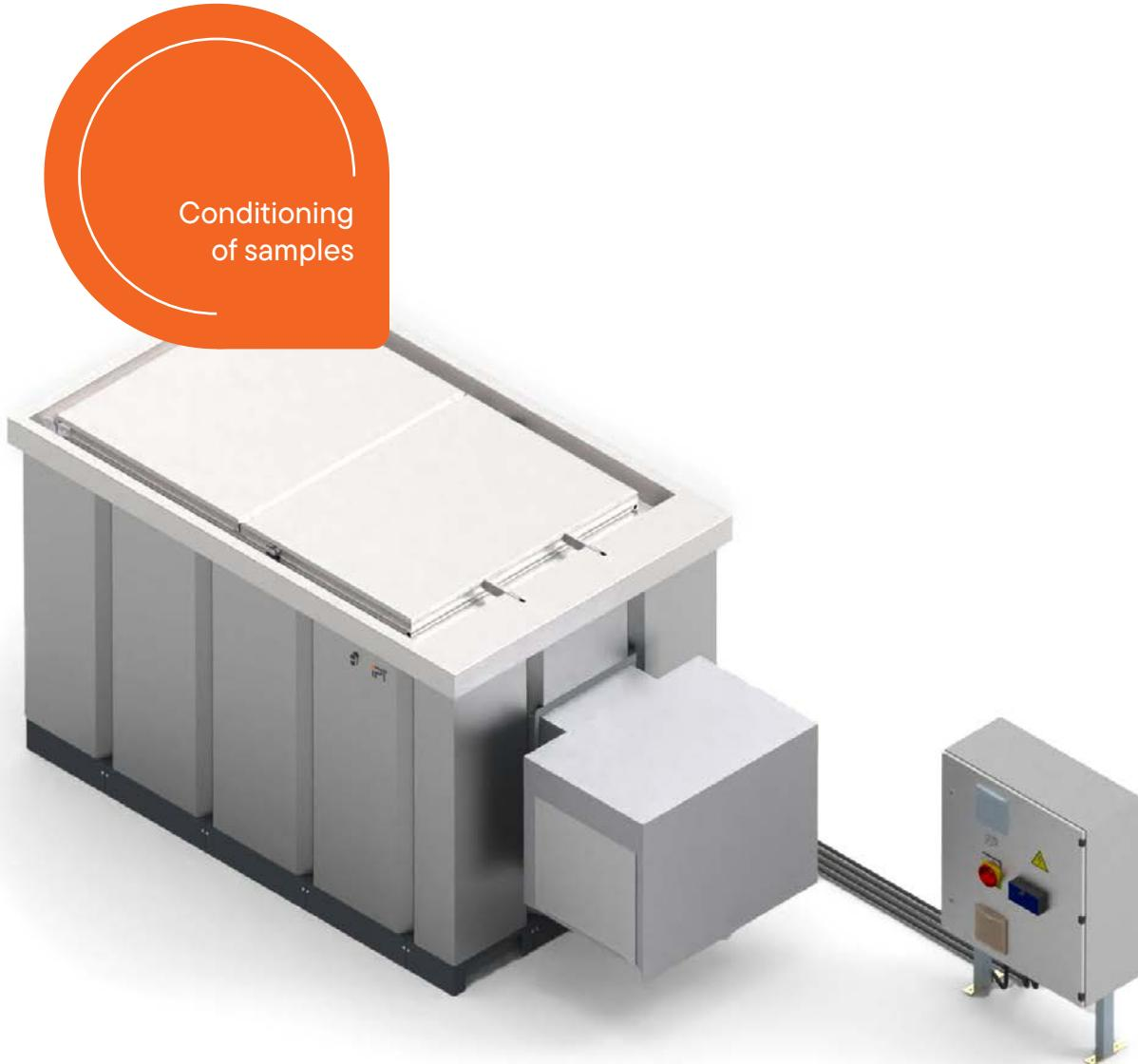
Impact and drop tests often require sample conditioning at a temperature of 0 degree Celsius. The zero degree test tank 1763 is suitable for holding samples and contains a cooling aggregate and a circulation unit.
