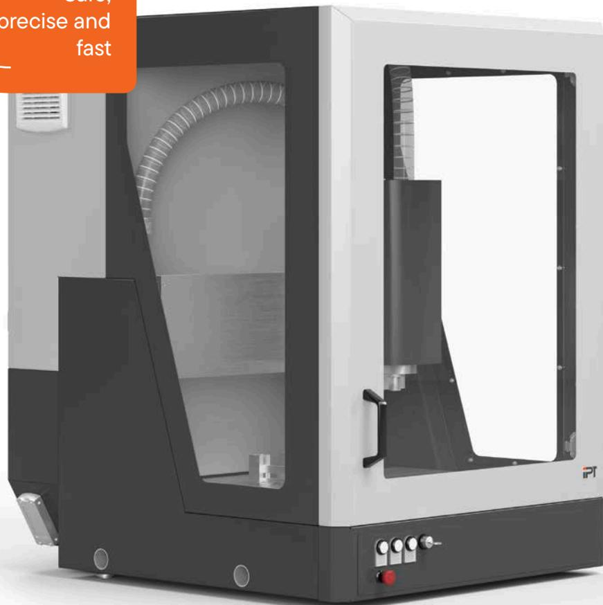
The CNC test bar milling machine enables bar-shaped plastic samples to be produced for tension, pressure, bending and flexural impact tests in accordance with a wide range of standards. The CNC milling machine is a table-top unit with electrically locking protective doors. Pre-configured machining programs for all common bar shapes and visualisation via Windows make it very easy to operate
