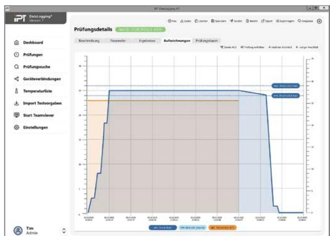
The purpose of this tester is to apply and maintain the correct hydrostatic pressure for internal pressure creep tests. Bursting pressure tests can also be optionally performed.
